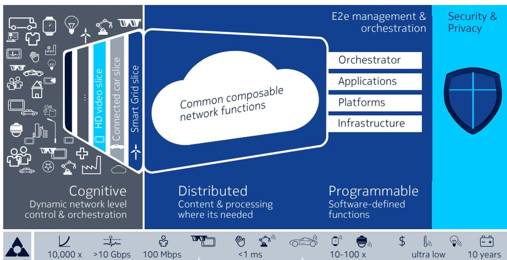
Figure 3: Network Slicing enabling Network-as-a-Service
