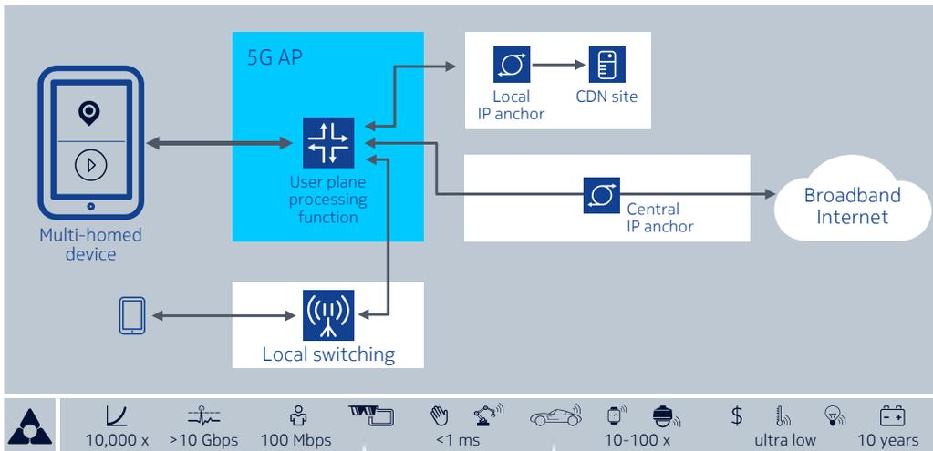
Figure 4: Service determined 5G connectivity model
